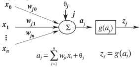
Where x0, x1, ... xn are inputs; wj0, wj1, ... win are weights;  $\theta j$  is the bias term; j is the unit; g(aj) is the activation function; and zj is the output.
