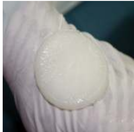
Fig. 1. The blend gel with good properties was provided after freeze-drying under vacuum at -56^{\circ}\text{C} .
